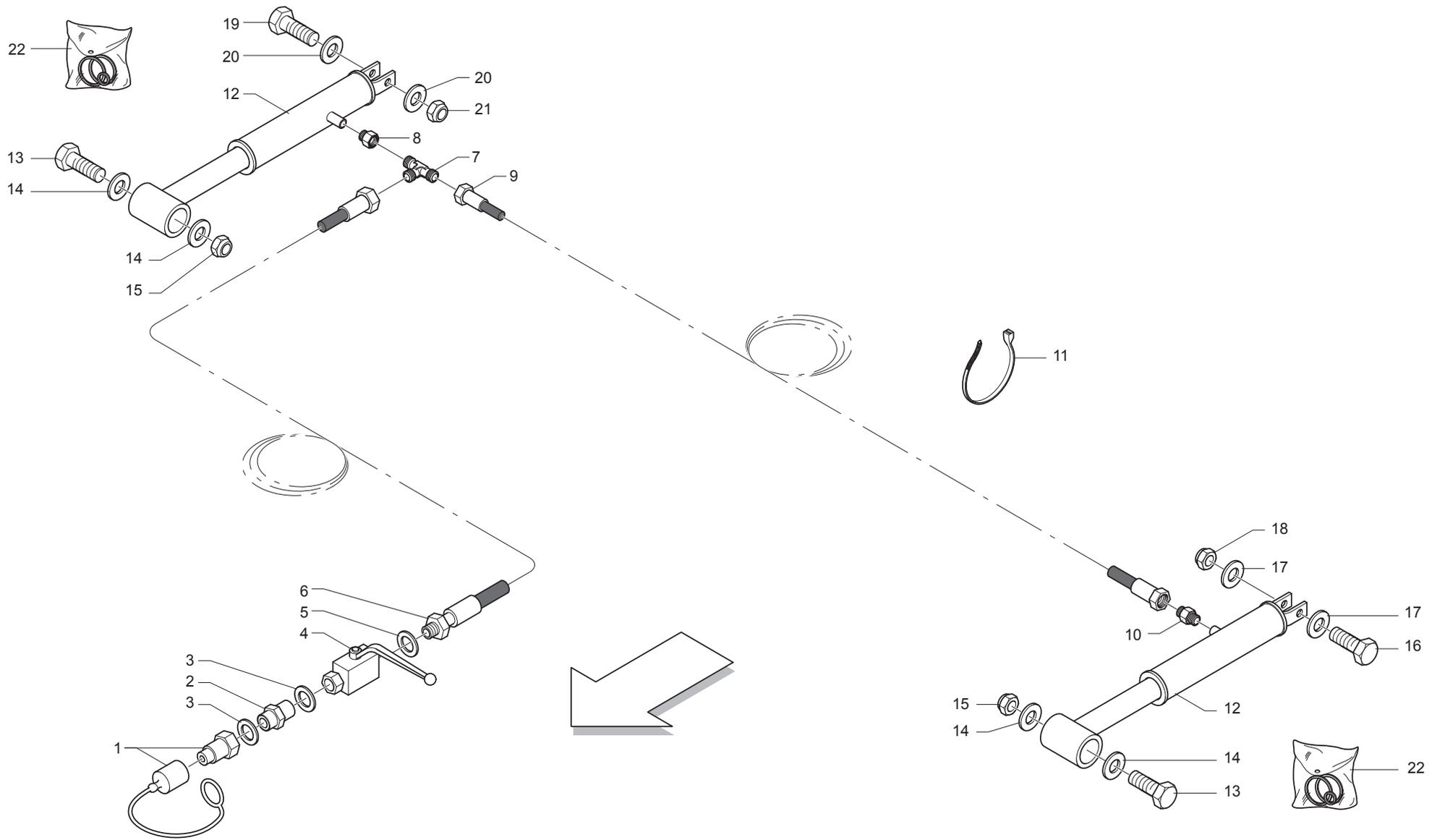
**IMPIANTO IDRAULICO PICK-UP
