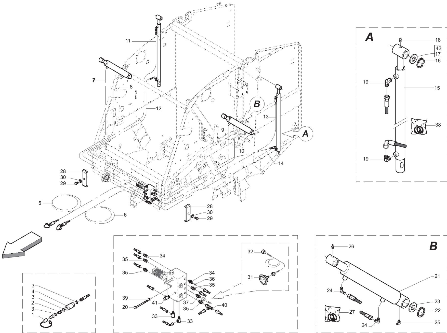
**IMPIANTO IDRAULICO MACCHINA
