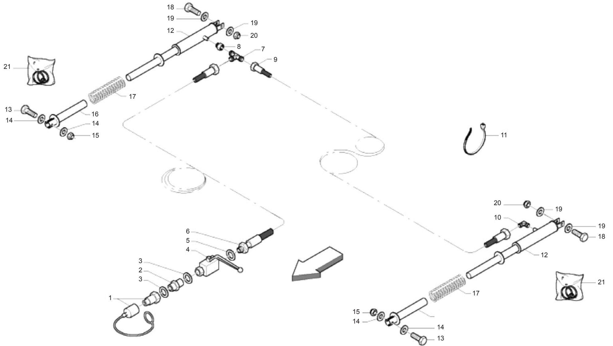
**IMPIANTO IDRAULICO PICK-UP CUT
