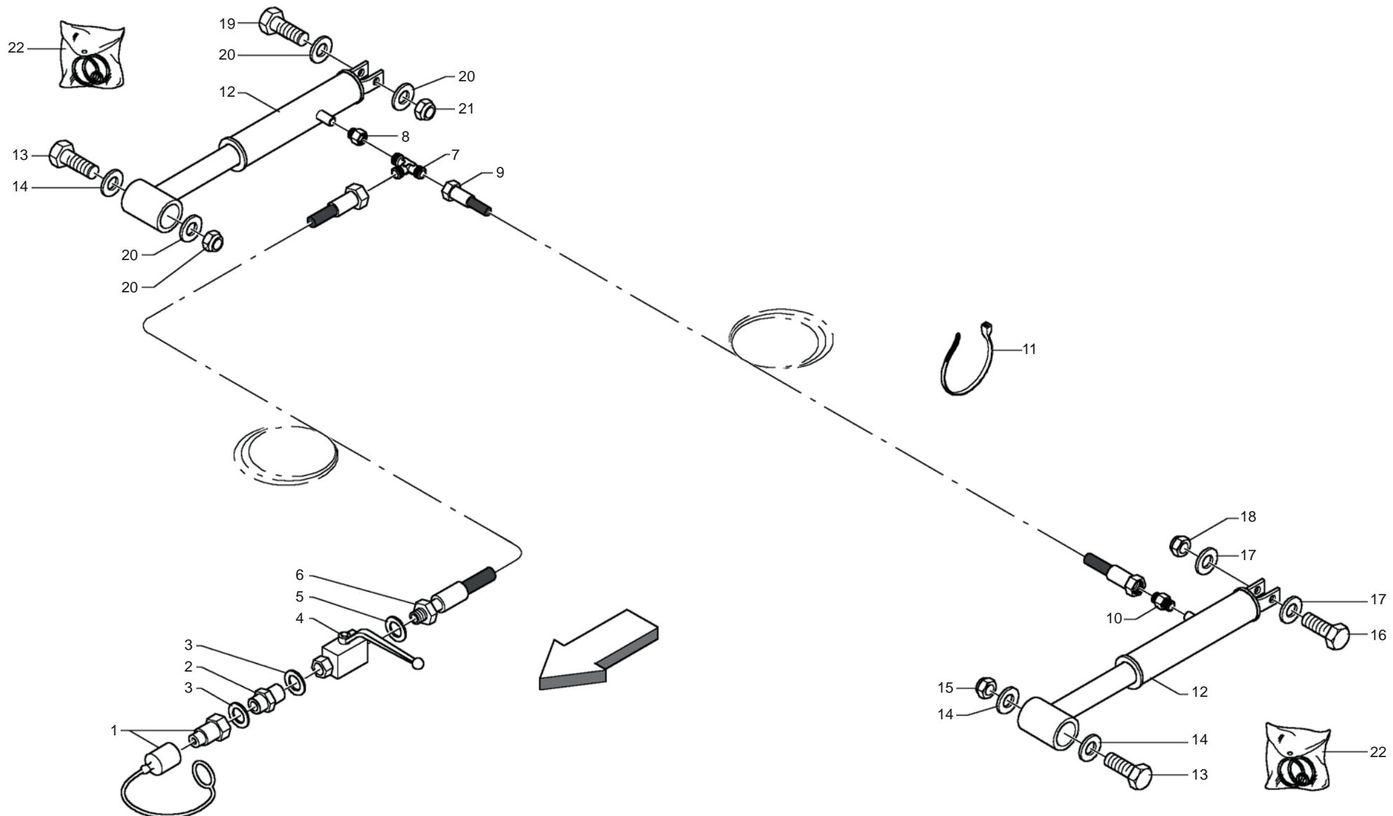
**IMPIANTO IDRAULICO PICK-UP**
