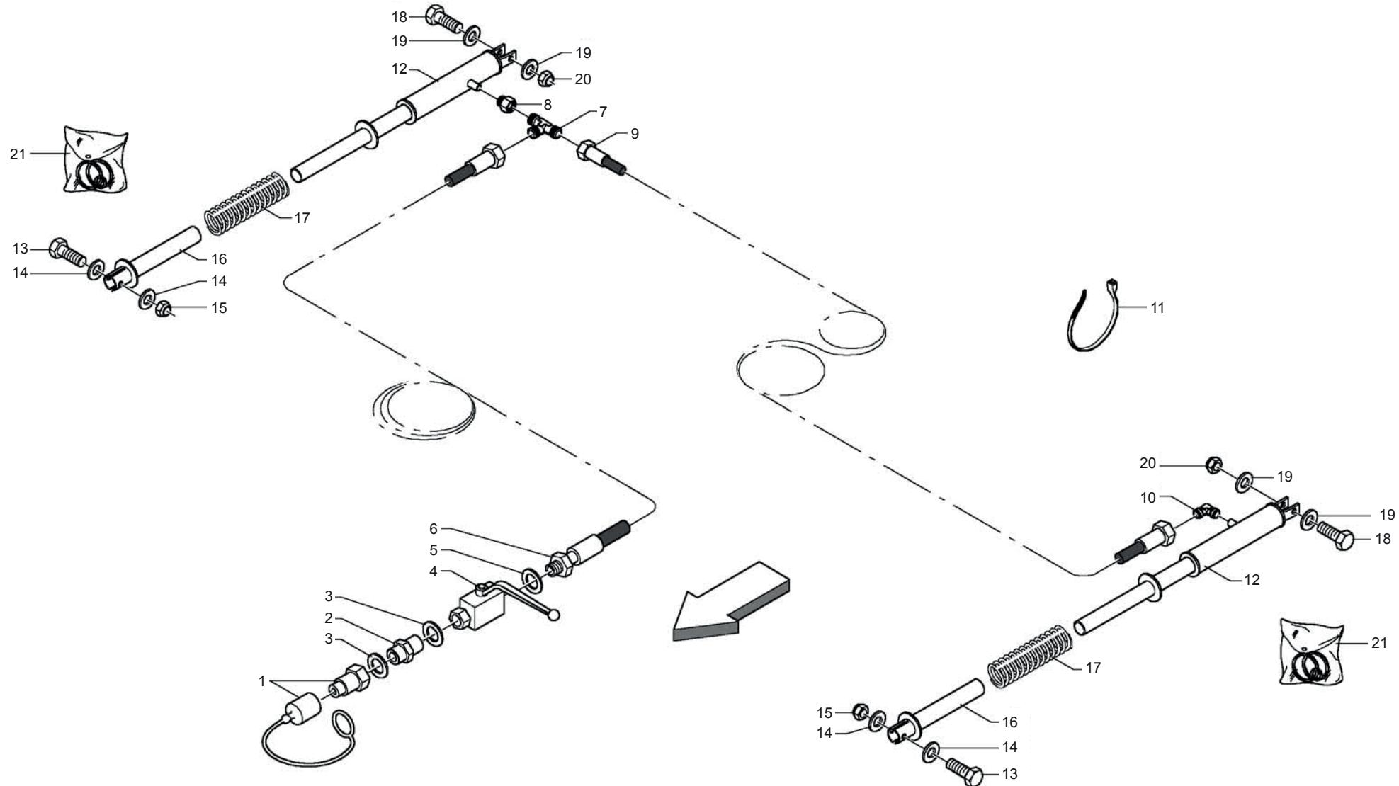
**IMPIANTO IDRAULICO PICK-UP CUT**
