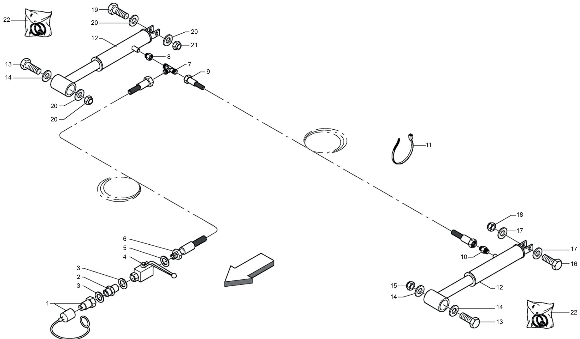
**IMPIANTO IDRAULICO PICK-UP**
