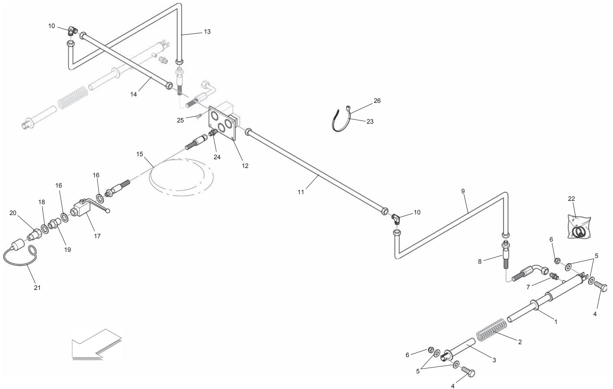
**IMPIANTO IDRAULICO PICK-UP
