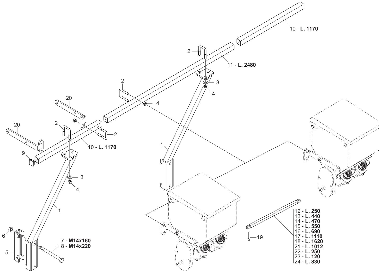
**SUPPORTI ED ASSI TRASMISSIONE MICROGRANULATORE**
