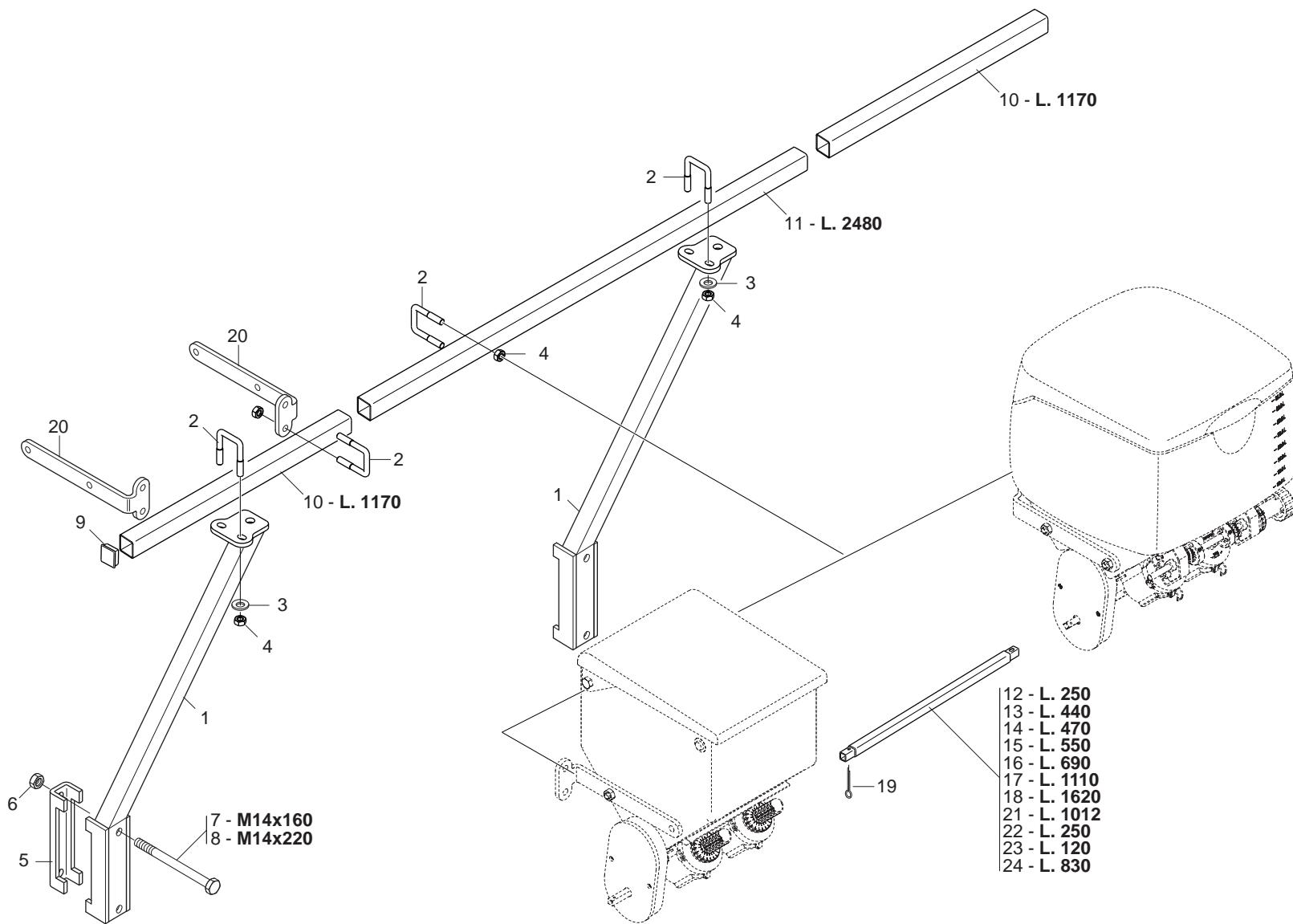
**SUPPORTI ED ASSI TRASMISSIONE MICROGRANULATORE**
