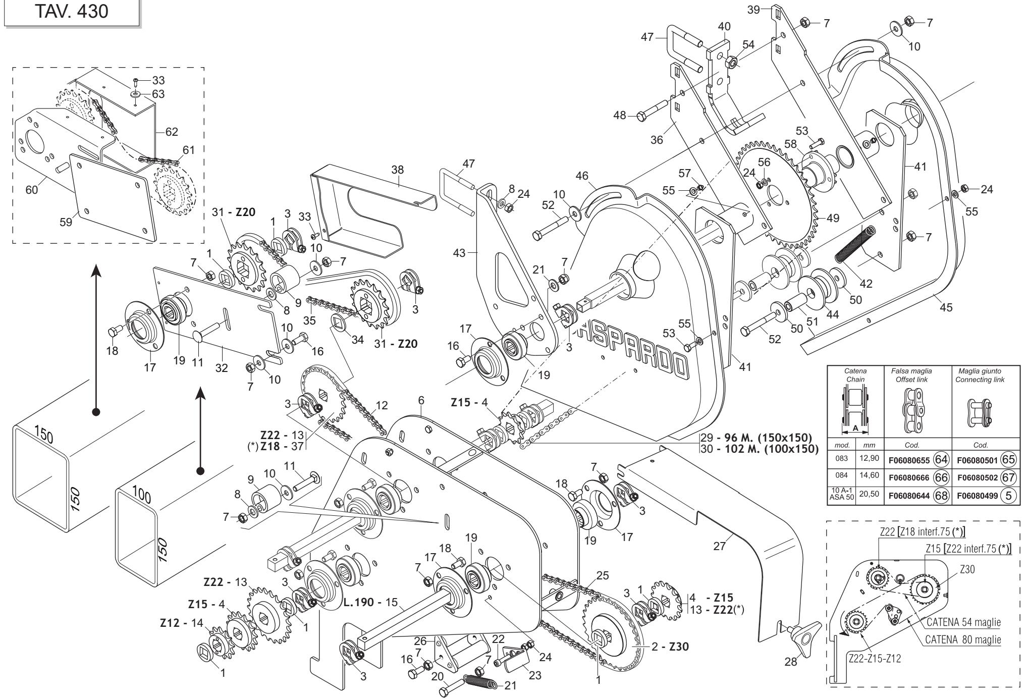
**TRASMISSIONE SPANDICONCIME E MICROGRANULATORE (45-50 cm)**
