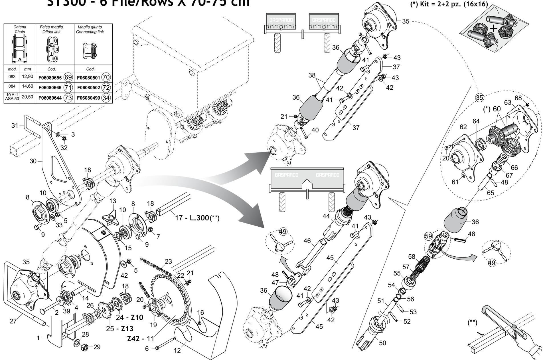
**TRASMISSIONE MICROGRANULATORE (6 file x70-75 cm)
