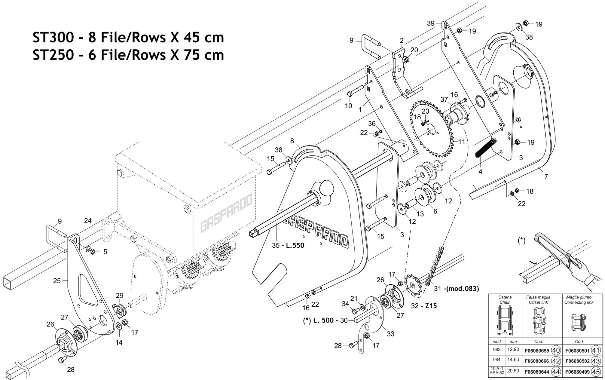
**TRASMISSIONE MICROGRANULATORE (8 file x45 cm)
