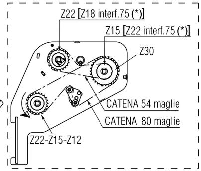
**TRASMISSIONE MICROGRANULATORE (7 file x50-60 cm)
