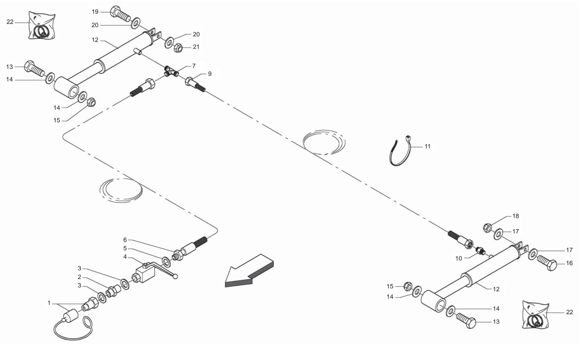
**IMPIANTO IDRAULICO PICK-UP
