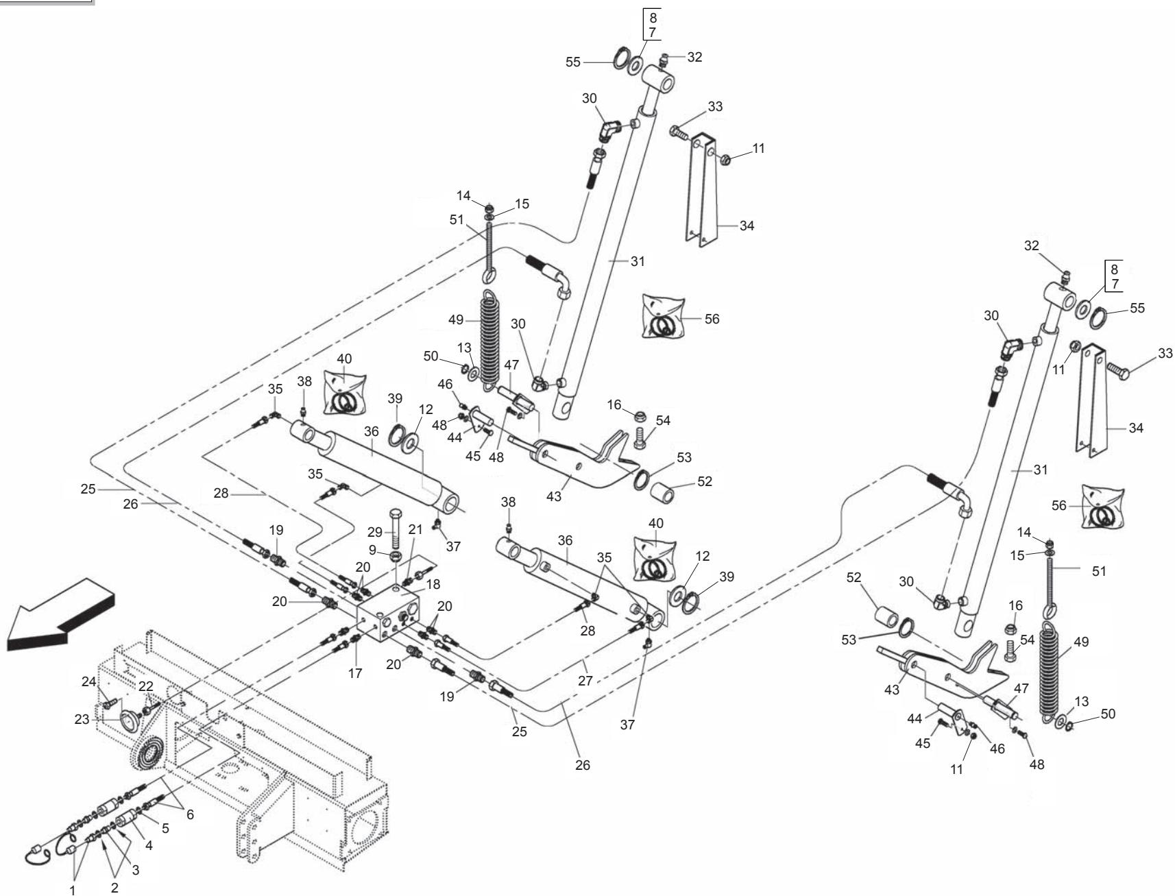
**IMPIANTO IDRAULICO MACCHINA**
