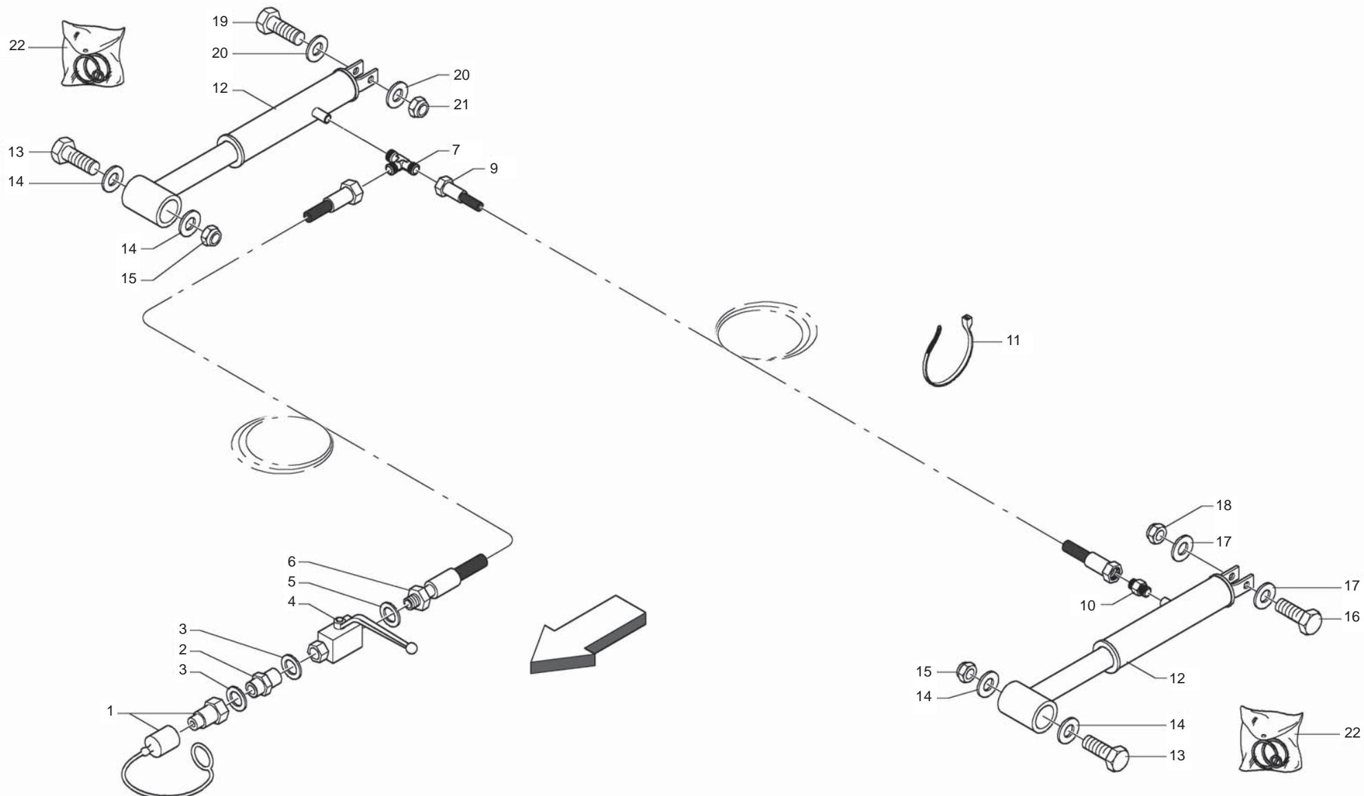
**IMPIANTO IDRAULICO PICK-UP**
