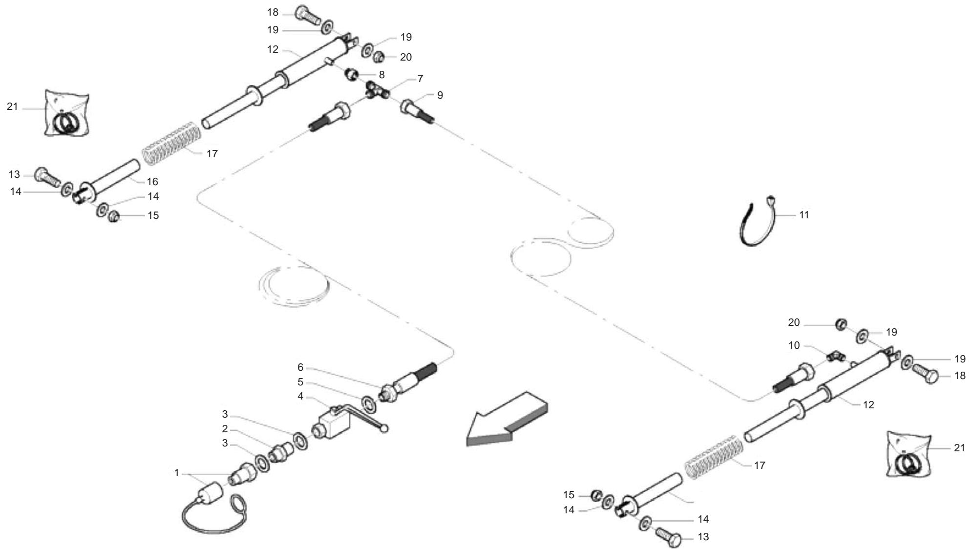
**IMPIANTO IDRAULICO PICK-UP CUT**
