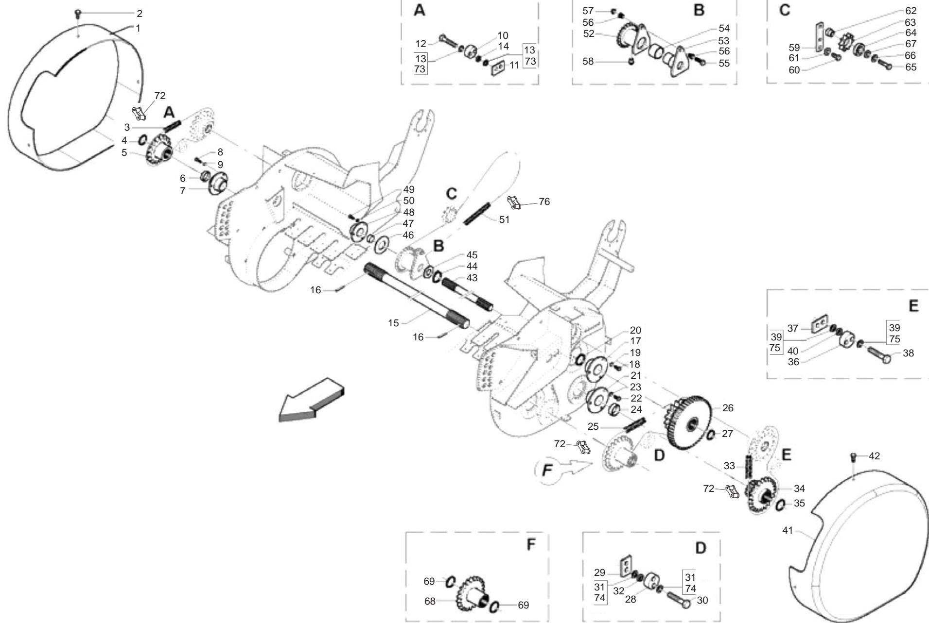
**TRASMISSIONE PICK-UP M CUT**
