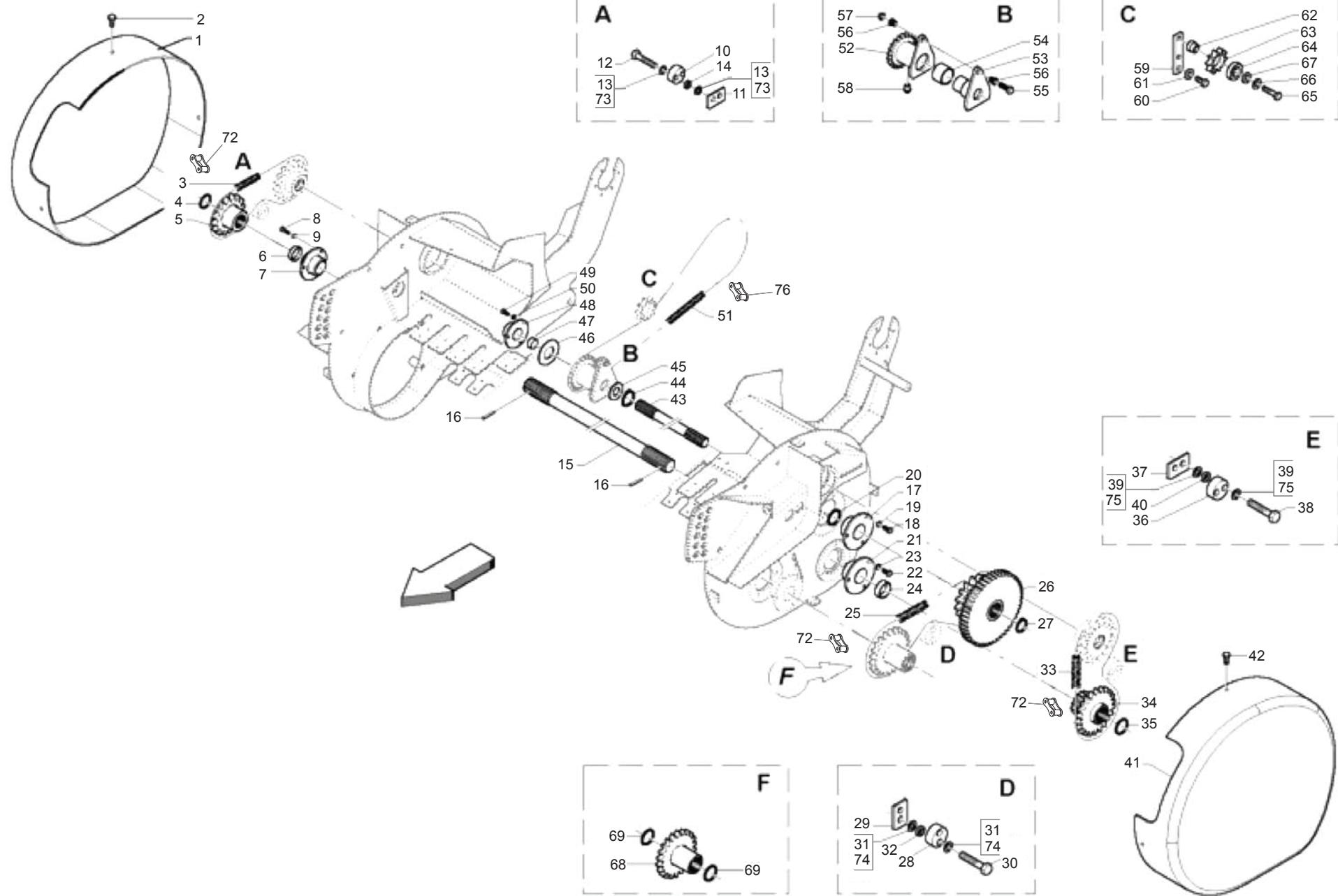
**TRASMISSIONE PICK-UP M CUT**
